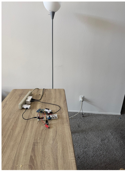
Left: The breadboard setup with the Qorvo ultra-wideband board connected to the nRF board Right: The setup in context with the lamp being controlled in the background.
